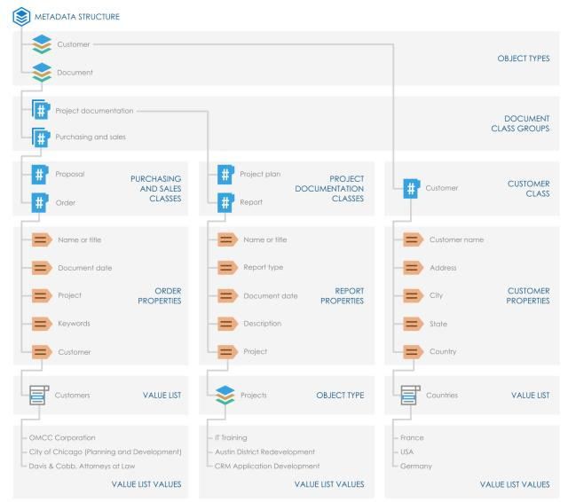
Figure 40: The vault metadata structure consists of object types, class groups, classes, property definitions, and value lists. The example above illustrates the hierarchy of a metadata structure that contains the Customer and Document object types and various classes for the two object types.
