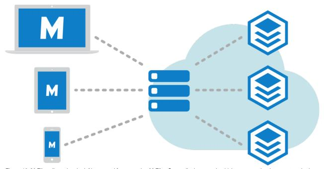
Figure 19: M-Files clients (on the left) are used for accessing M-Files Server (in the center), which manages the document vaults (on the right).
