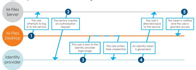
Figure 21: Authentication flow in a federated authentication system.
