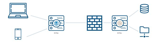
Figure 69: A Ground Link proxy lets a vault connect to private repositories, such as network folders, without a direct network path.
